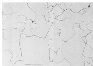
Fig. 3. Alumina containing magnesia fired in hydrogen for 21 hours at 1850°C and then for 23 hours at 1900°C; density, 3.97 g per cm<sup>3</sup> [X255.]
