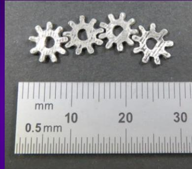
~ 50 micro-gears by one SPS run
