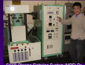
Spark-Plasma Sintering System (MPS) Dr. Sinter 515S at SDSU. Max Load 50kN, max current 1500 A
